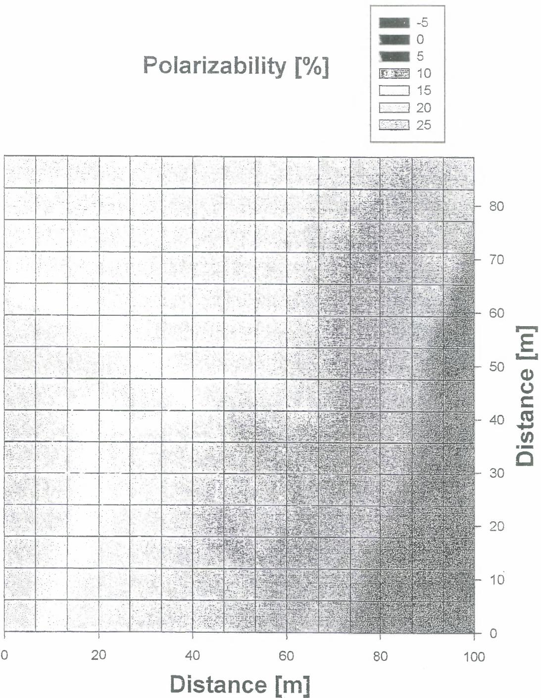
Fig. 20 Contoured plan of area 1 showing the changes in polarizability (hydrocarbon content) across the area
