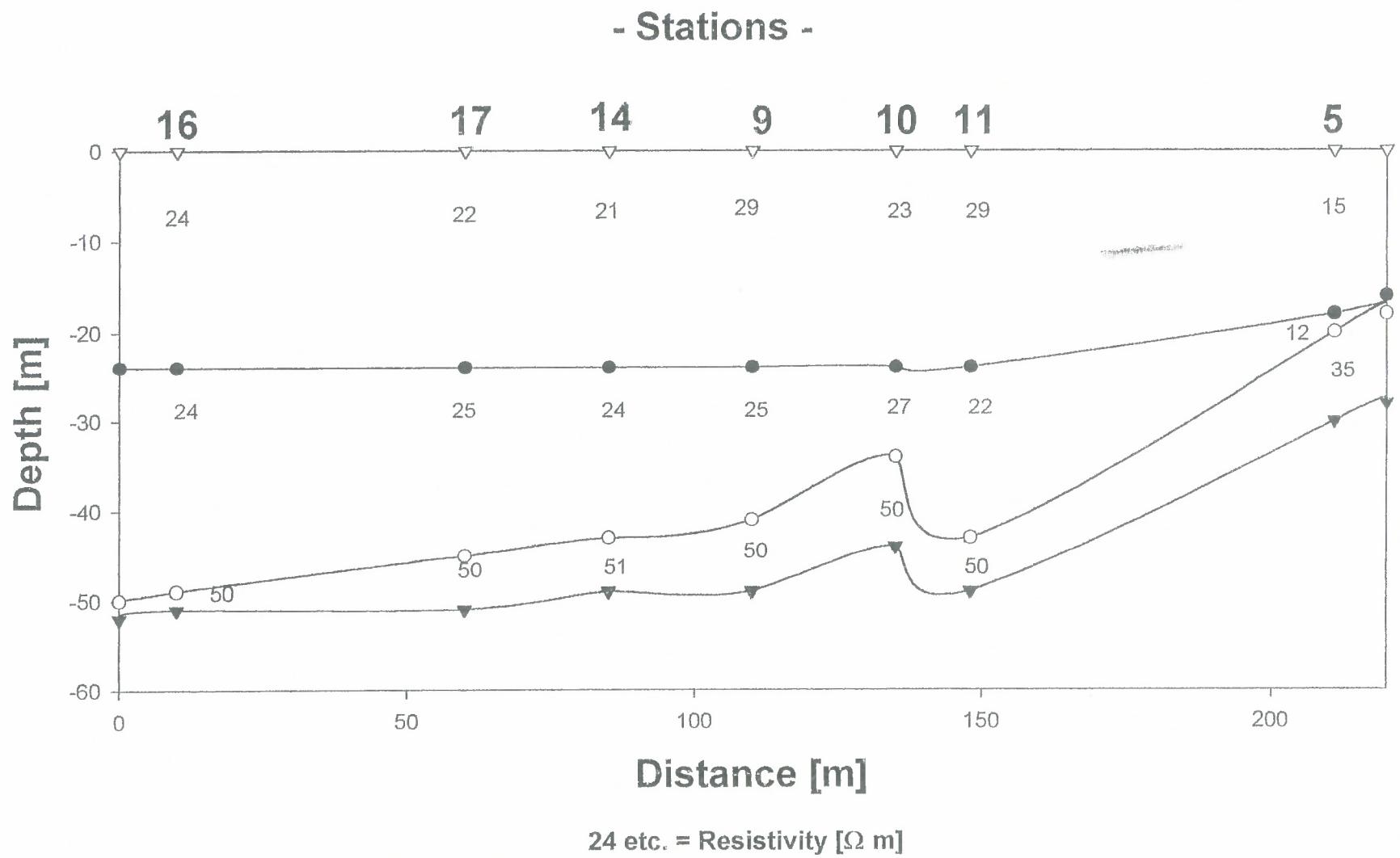
Fig. 19 Geoelectrical cross section showing the distribution of resistivity values for the stations of area 1
