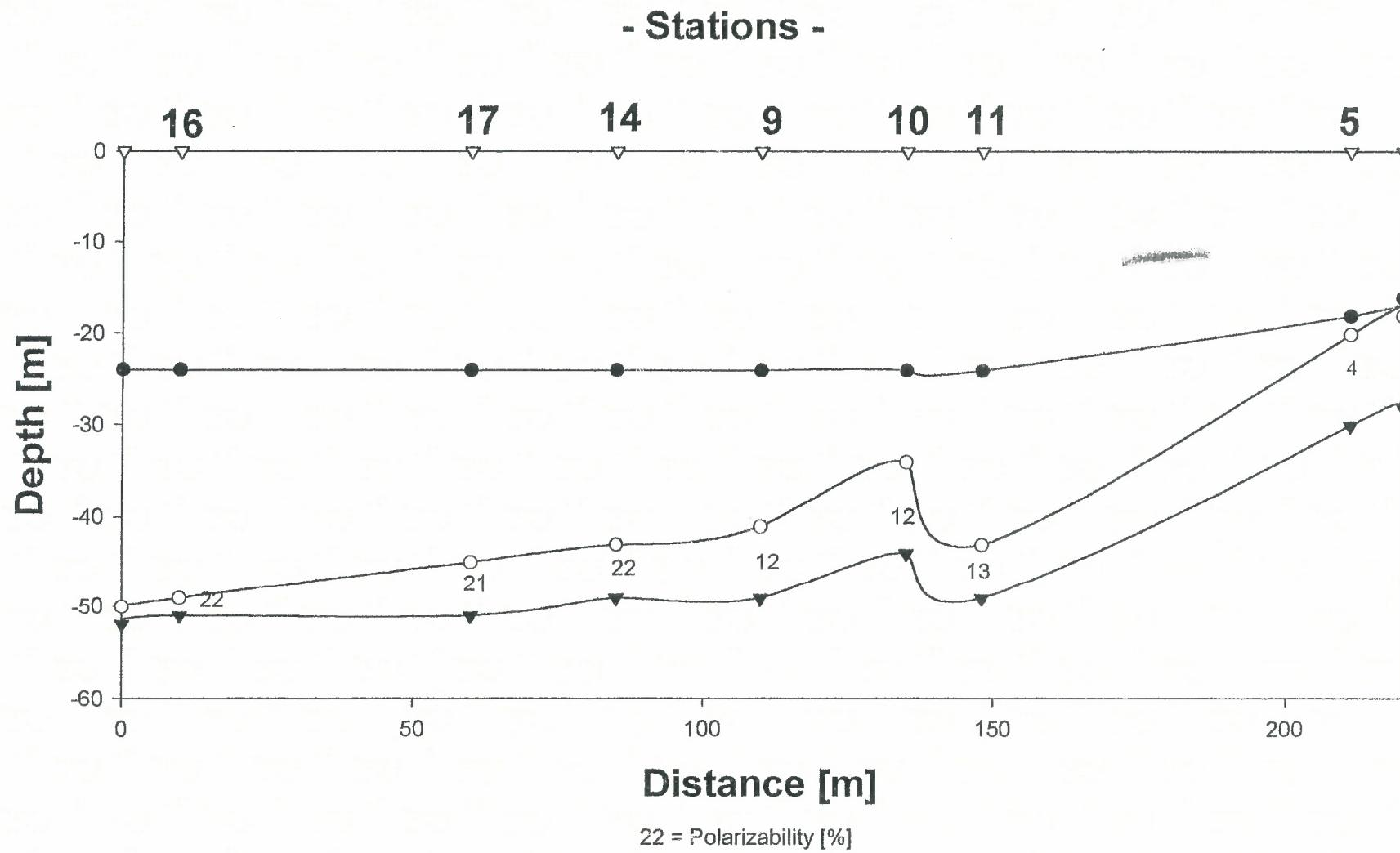
Fig. 19 a Geoelectrical cross section showing the distribution of polarizability values for the stations of area 1. Highest polarizability is correlated to high hydrocarbon pollution
